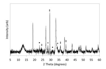
Fig. 7. Powder XRD pattern of zinc-exchanged LS-4 (key:  $\text{Li}_2\text{SiO}_3$  – unmarked;  $\text{Ca}(\text{OH})_2$  – \*;  $\text{Ca}(\text{CO}_3$  – \$\frac{1}{2}\$;  $\text{Li}_2\text{CO}_3$  – \$\frac{1}{2}\$
