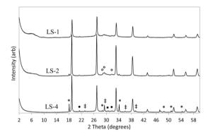
Fig. 1. Powder XRD data for the hydrothermal reaction products of waste glass and aqueous lithium hydroxide (key: Li<sub>2</sub>SiO<sub>3</sub> – unmarked; Ca(OH)<sub>2</sub> – \*; CaCO<sub>3</sub> – ‡; Li<sub>2</sub>CO<sub>3</sub> – •; Ca<sub>5</sub>Si<sub>6</sub>O<sub>16</sub>(OH)<sub>2</sub>·4H<sub>2</sub>O – °)
