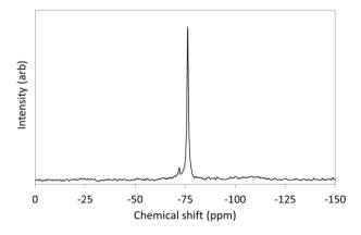
Fig. 4. <sup>29</sup>Si MAS NMR spectrum of the hydrothermal reaction products of waste glass and aqueous lithium hydroxide
